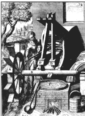
Water-powered fulling stocks
